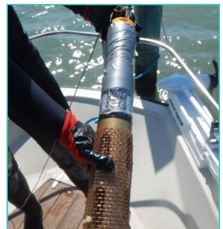
YSI EXO3 data sonde before its first deployment in Estero Bay Aquatic Preserve.
