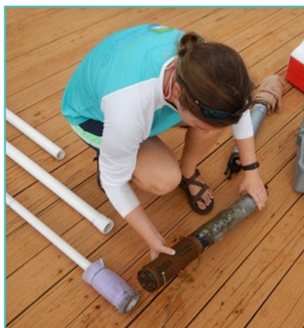
Estero Bay Aquatic Preserve water quality technician prepares to inspect a retrieved data sonde and deploy another instrument.
